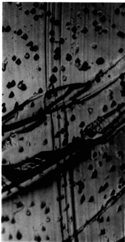
Fig. 6. Stratigraphical etch pattern on a (10\bar{1}0) cleavage face of apatite ( \times 80 ).
