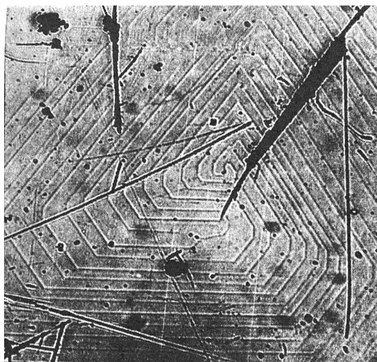
Figure 5. Reflected light photomicrograph of a complex growth spiral on a \{100\} face of an apatite crystal from Sulzbachtal, Austria. The horizontal steps run in the [001] direction. [Used by permission of Macmillan Publishers Ltd., from Amelinckx (1952) Nature , Vol. 170, Fig. 1, p. 760.]
