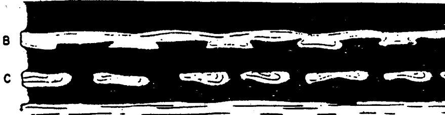
Fig. 125. Scheme showing the genesis of load structures on the lower surface of a sand layer resting on a mud layer (black)
