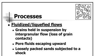
Flow "freezes" from bottom up as it slows and sediment is redeposited
